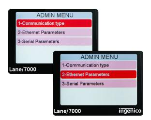
**2E)** Select "Ethernet Parameters", then "IP Configuration", then "DHCP activation" and then select "Off" and press the green "Enter" key.
